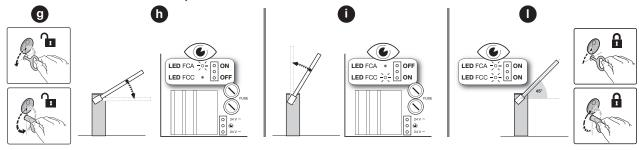
Note - In order to exploit the slowing down function most effectively, it is necessary that the limit switch triggers at about 20° before the mechanical stopping point is reached; if necessary adjust the two cams to set the desired point.
