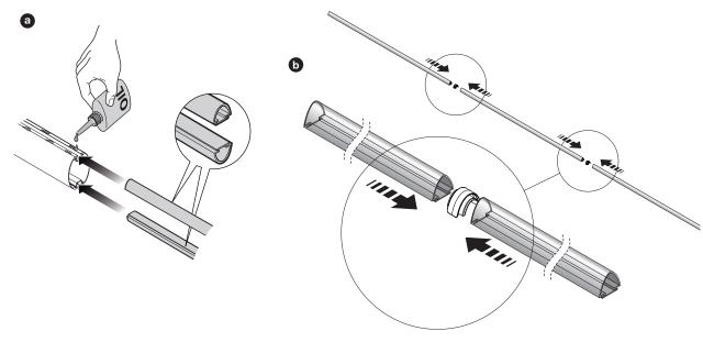
$\boldsymbol{c}$  - insert the joint for the rubber impact protector and repeat for the other pieces Note - The rubber impact protector can protrude about 1 cm from the end of the aluminium profile
