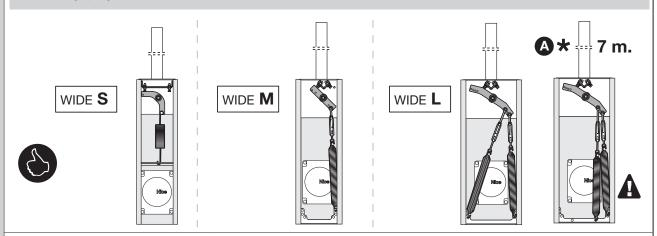
▲★ Only with 7 m boom place the balancing springs as shown in Figure "A"
