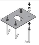
**04.** Cast the concrete to secure the foundation plate
