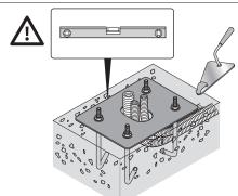
**05.** Wait until the concrete hardens (usually at least two weeks) and then remove the 4 upper nuts of the anchors
