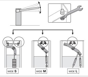
**13.** Adjust the balancing of the boom, according to the model purchased:
