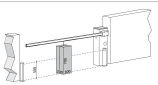
If the test is on two pairs of photocells, the test must first be performed individually for each pair of photocells using 1 testing block and then repeated using 2 testing blocks.
