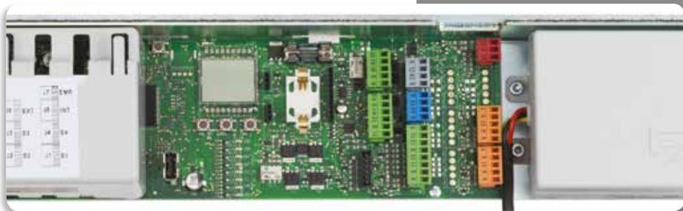
CONTROL UNIT WITH SWITCHING POWER SUPPLY
