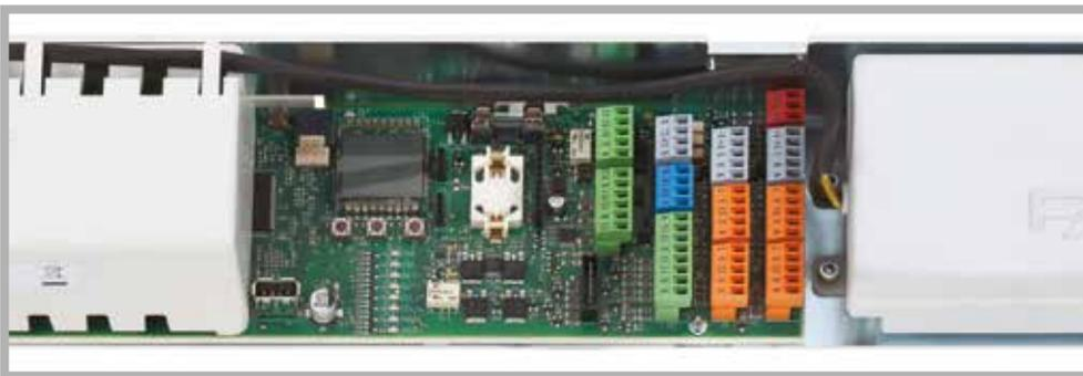
**2** Control unit with switching power supply
