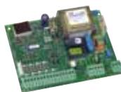
578D electronic control unit (remote installation)
